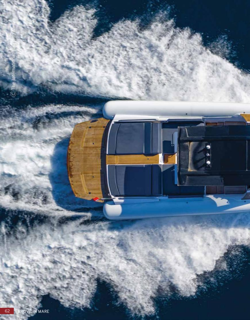
I have already tested other Magazzù yachts, I know that the shipyard represents the highest experience in the design of stepped hulls but this....this is really a superhull.. And, indeed, as the speed increases by just 400rmp more, we're sailing at more than 20 knots. At this speed, we're consuming just 60 l/h in total, which clearly suggests that this is an extraordinary hull with minimal resistance to advancement, especially
